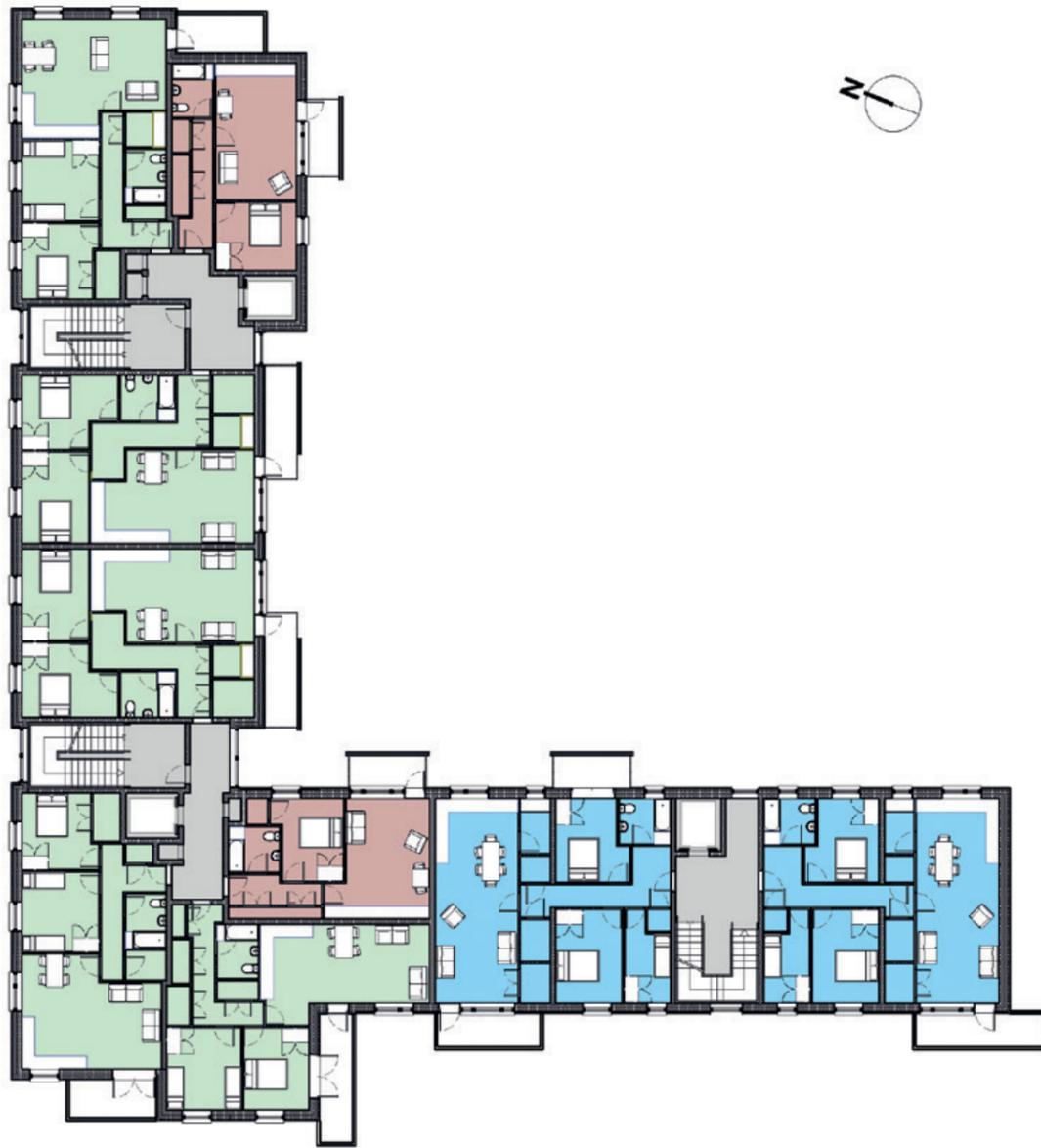
Typical upper level floor plan, with colour coding of 1 Bed, 2 Bed, and 3 Bed apartment typologies.
