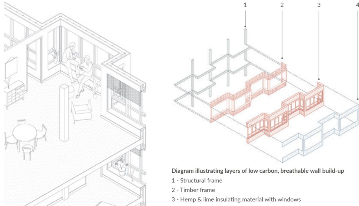
Diagram illustrating layers of low carbon, breathable wall build-up
