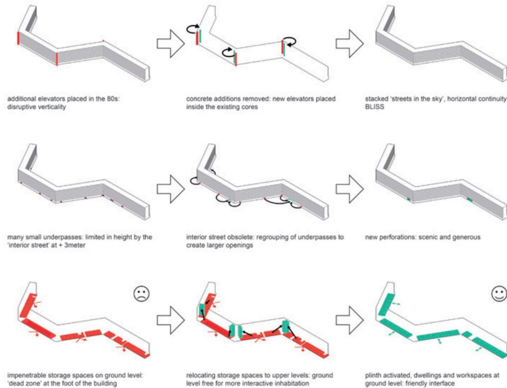
Diagrams illustrating existing conditions/challenges within block, and refurbishment strategy with key alterations completed.
