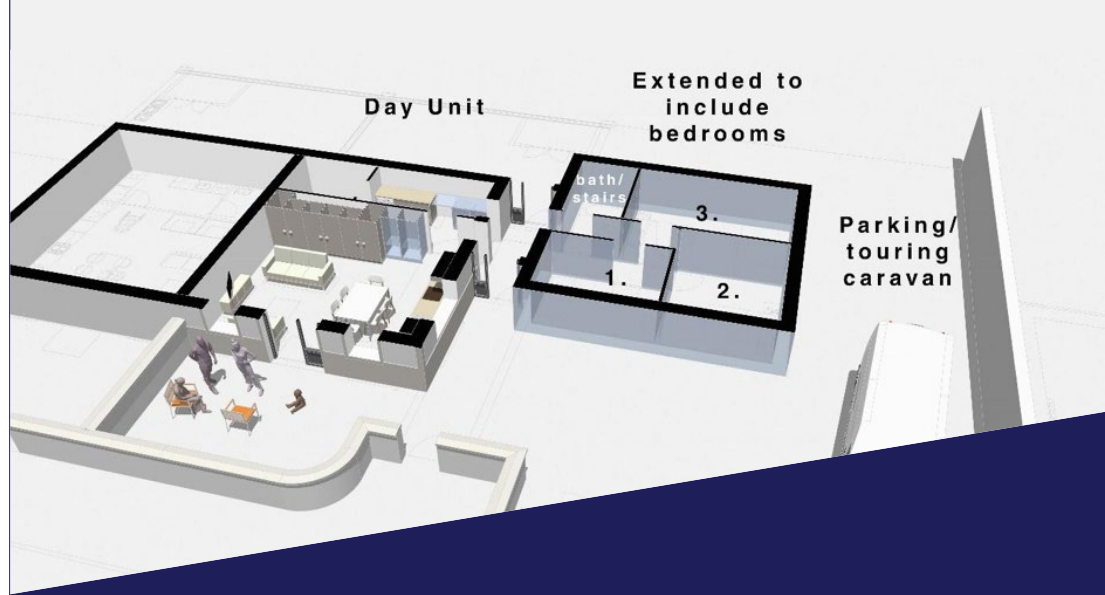
Figure 6: Day unit study, indicating where required fire safety offset distance is utilised to allow future expansion of the day house to provide sleeping accommodation.
